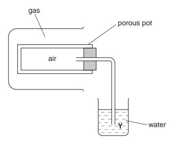
A beaker containing the gas was placed over the porous pot.
